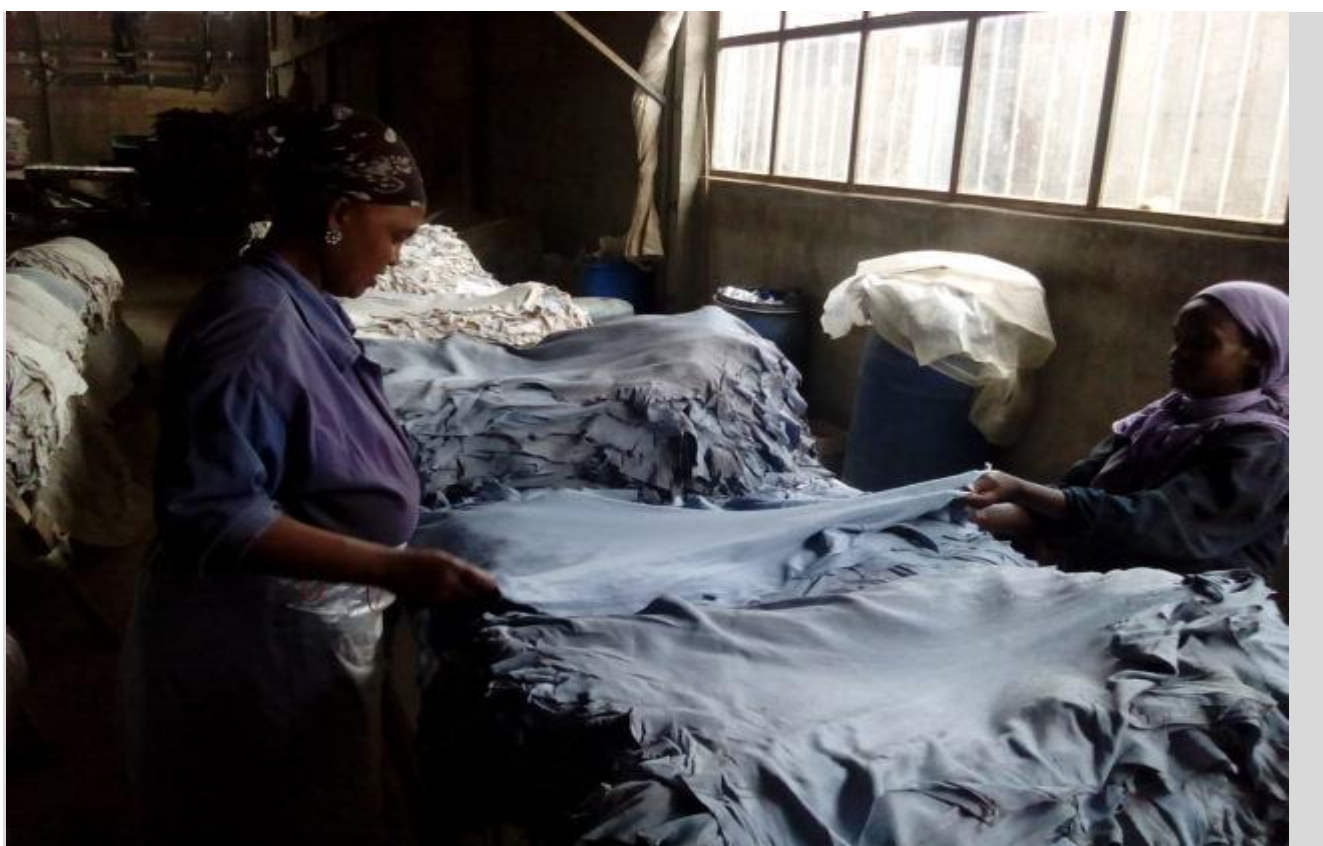
Figure 1 - Observation of defects and grading wet blue goat skins in properly prepared and lighted point at Gelan tannery in Modjo
